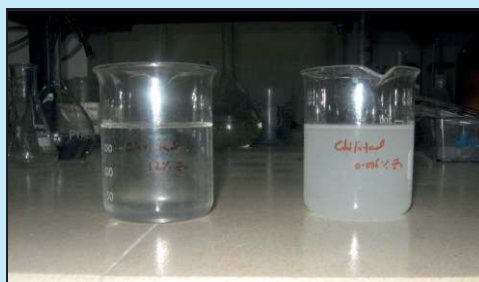
Good quality Zinc sulphate monohydrate and adulterated Zinc sulphate, monohydrate solution
